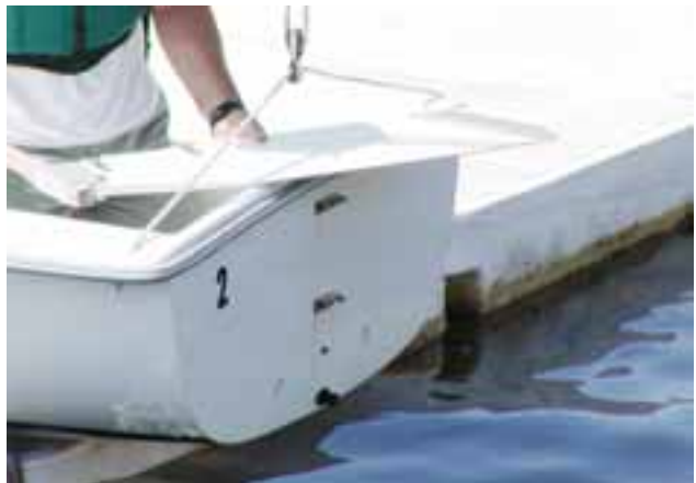
22. Provided that the tide is not extremely low you may put on the rudder . Pass the rudder under the traveler (the bridle which controls the sideways movement of the boom). If the tide is low you will put the rudder on after the boat is brought to the windward side of the dock.
